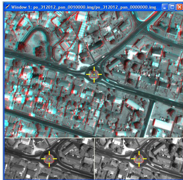
GeoEye-1 Stereo Imagery in LPS, displayed in anaglyph mode
